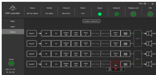
When switched to 70 V mode, DP-N (F) models have Peak Limiter and RMS Limiters set automatically. Only the HPF needs setting in the EQ section.
