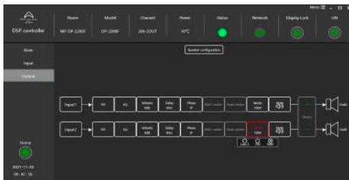
When switched to 100 V mode, DP-N (F) models have Peak Limiter and RMS Limiters set automatically. Only the HPF needs setting in the EQ section.
